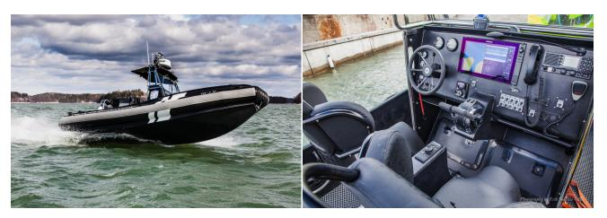
Steering consoles and other interior details are easy to customize to the needs of the operator. Polyethylene boats need no molds. All parts are water cut and welded.
